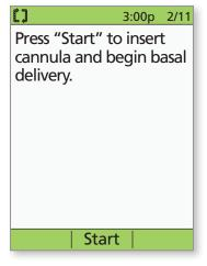
+ Press **Start**. The Pod automatically inserts the cannula and delivers a prime bolus to fill the cannula with insulin. It takes a few seconds to complete this process. Release the skin after the cannula inserts.
